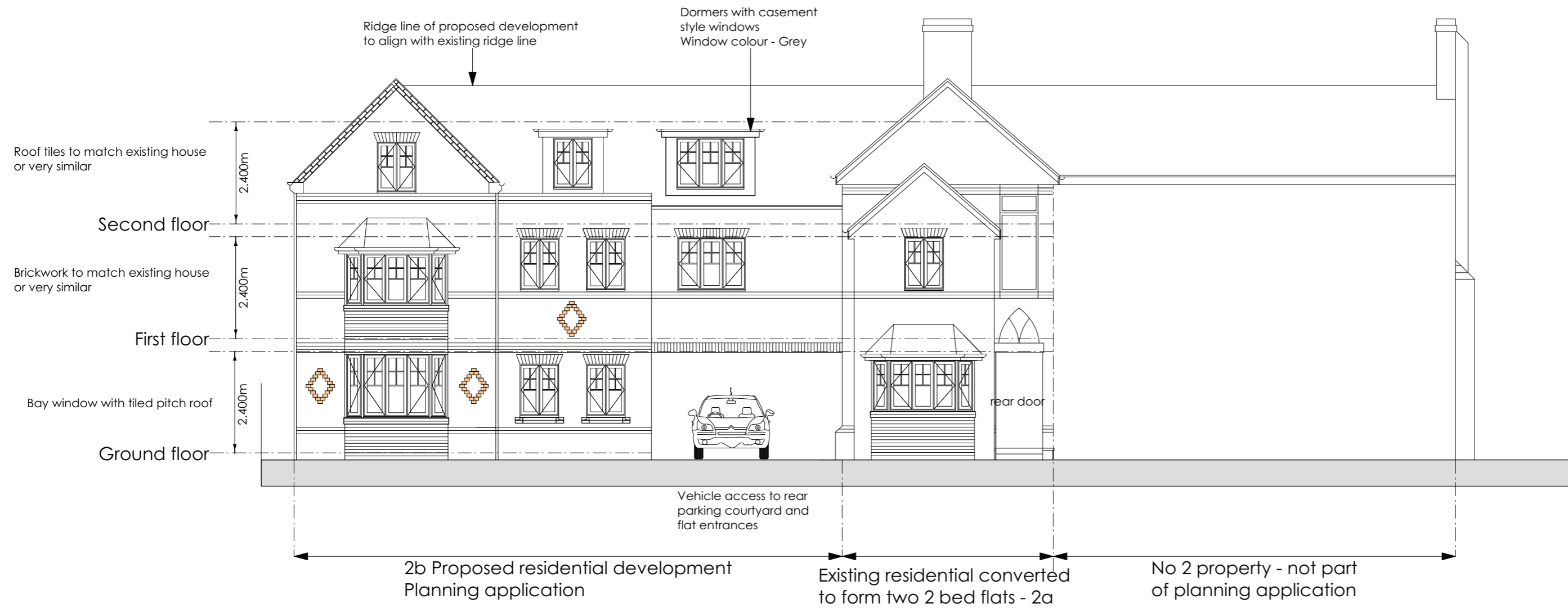
Elevation to rear Scale 1 : 100
